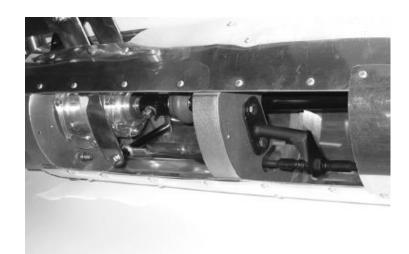
Cut the tail boom skin to clear the pitch actuator arms as shown, removing no more than necessary.
